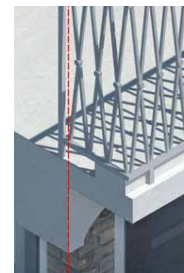
Fig 5.8.22 Balcony detail. Projection and structural upstand. (Red = wall line).
